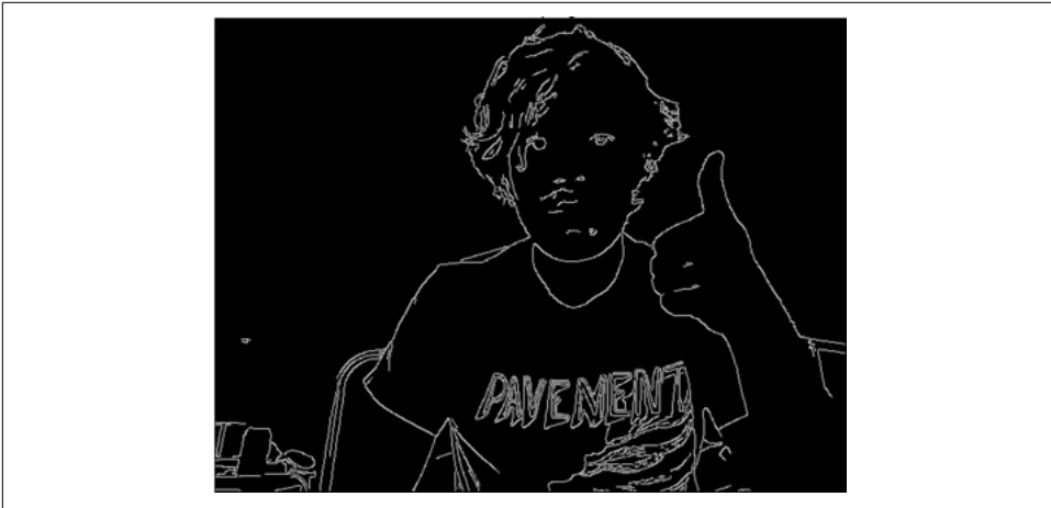
Figure 4-6. Edge detection algorithms find boundaries between areas with different colors or intensities
