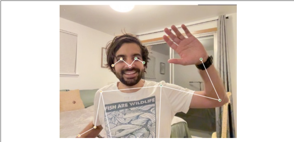
Figure 4-9. Pose estimation identifies key points on a human body, the position of which can be used as input for other processes
